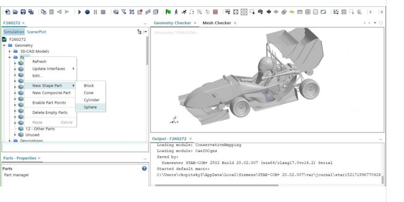
To find where the surface intersects itself, open the Geometry Checker, then go to Gemoetry -> Parts (Right-Click)-> New Shape Part -> Sphere
