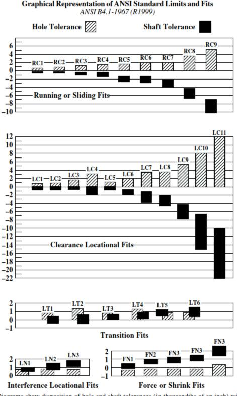
Diagrams show disposition of hole and shaft tolerances (in thousandths of an inch) with respect to basic size (0) for a diameter of 1 inch.
